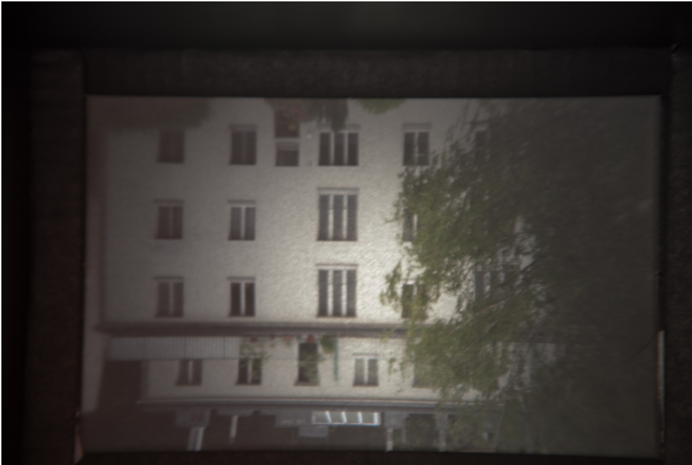
Fig. 30. The image on the matte paper is sharp in center, inverted, with geometrical aberration as we look farther from the center, the intensity of light is dimming from center towards the corners; somehow resembles with the cone of attention what we present in human vision, but also we understand, why retina is a hemispherical surface and not a planar one.
